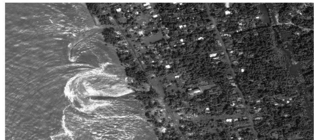
Fig. 12. Evolution of the 2004 Indian Ocean tsunami near the coast of Sri Lanka: the form changes from the wall of water (low part), through the breaker to the localized jet (upper part)
